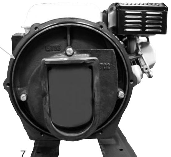
8. Install the pump body (15712) onto the rear bracket aligning the pump body with the dowell pins on the rear bracket. Secure the pump body to the rear with six bolts (12715A) and (6) lock washers (V10118).
