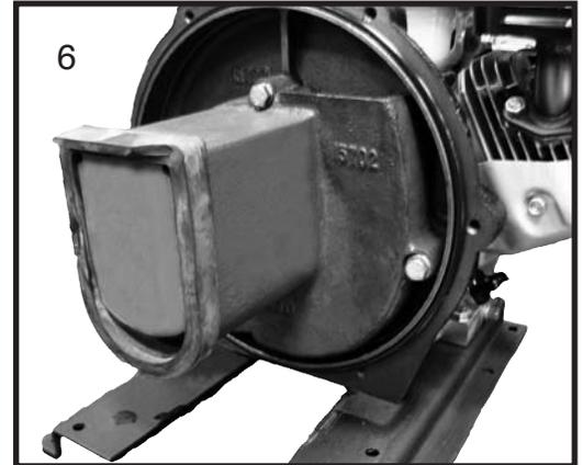
7. Place the main pump body o-ring (12719A) on the outside flange of the rear bracket. The gasket should be aligned with and placed over the two dowell pins on the rear bracket. The gasket may be lubricated with chapstick or petroleum jelly. Lubricating the gasket in this manner will help the parts not to stick to the cast iron parts it is sealing against.
